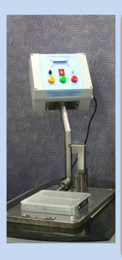
Locking Load Indicator system used to find out mechanical defects in cooker i.e. wrong angular position of cooker's handle.
